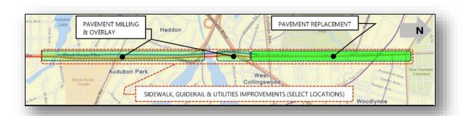
approximately M.P. 8.56 to 9.80), a Road Diet and Complete Streets enhancements (from approximately M.P. 9.80 to 10.75), ADA accessible sidewalks, approximately 8 signalized intersections, bicycle lanes (from approximately M.P. 9.80 - 10.44), improved bus stops, at-grade rail crossing safety improvements, guiderail upgrades, utility relocations, upgraded stormwater management infrastructure, and Intelligent Transportation System (ITS) deployment.
